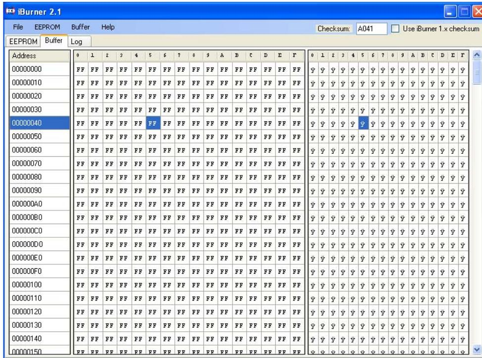
Buffer operations are executed from the *Buffer* tab and the *Buffer* menu. The *Buffer* tab has two main panels; the left panel displays the contents of the buffer in hexadecimal while the right displays the same information as printable ASCII characters (if possible). The contents of the buffer may be edited manually by double-clicking on any cell and entering a new value (either hex in the left panel or ASCII in the right panel).
