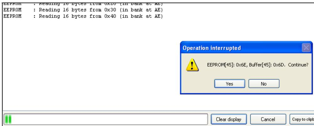
Clicking the *Verify* button or *Verify* from the *EEPROM* menu initiates a comparison between the contents of the EEPROM and the buffer. If any bytes are found to be different, the user is prompted to stop checking or continue. The information is logged as it is processed, including user decisions.
