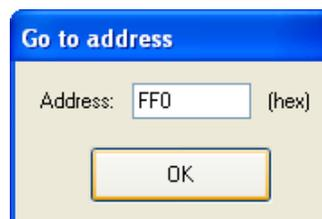
The *Go to address* operation simply moves the buffer view such that the user can see and edit the memory at the desired address.
