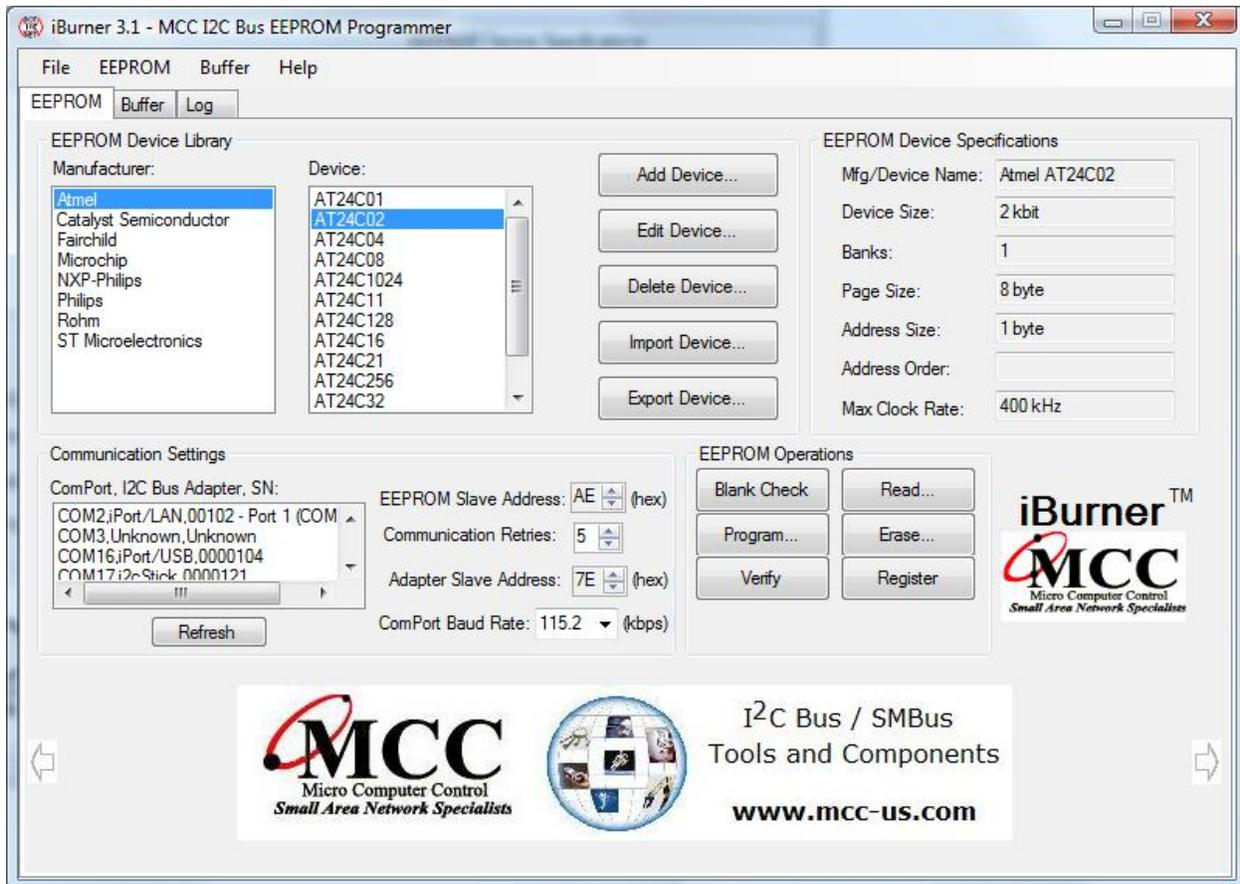
When iBurner is first started, you will see a window like that above. There are three tabs; the *EEPROM* tab is used to select an EEPROM and provide iPort configuration settings, as well as accessing some common actions. The *Buffer* tab provides a display of the current memory buffer upon which work is being done. Reading the EEPROM will read data into this buffer, and programming the EEPROM will write data from this buffer. The *Log* tab displays information on current and past operations.
