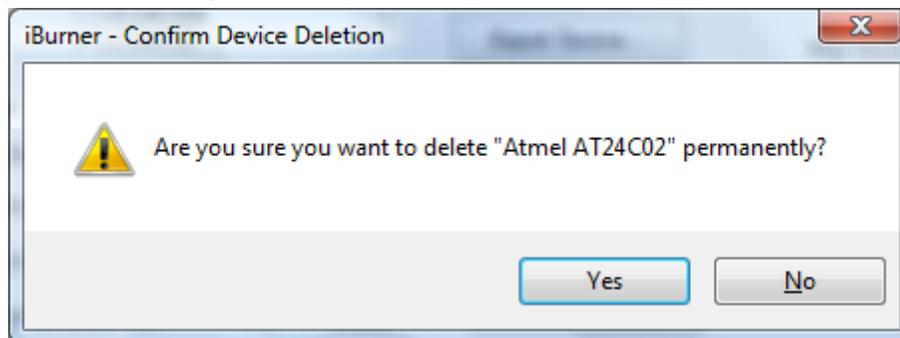
Devices can be removed from the device library by selecting the manufacturer and device and clicking the *Delete Device* button, or *Delete device* from the *Device Library* submenu of the *EEPROM* menu. A dialog box is displayed to confirm the removal.
