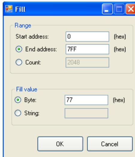
The *Fill* operation fills some portion of the buffer with data; either a repetition of a single byte value or a single instance of an ASCII string. The fill range can be described by a start address and either an end address or a count of bytes to be filled. The start address defaults to the address of the currently selected byte in the buffer and the end address defaults to the last address in the buffer (similarly, the count defaults to the total size of the buffer).
