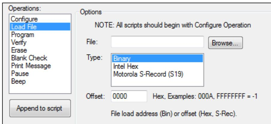
The “Load file” operation allows you to load a file into the buffer at a particular offset. The Script Creator supports the same files as the iBurner application. Click “Browse...” to select the file, choose the proper file type and offset, and click “Add to script”.
