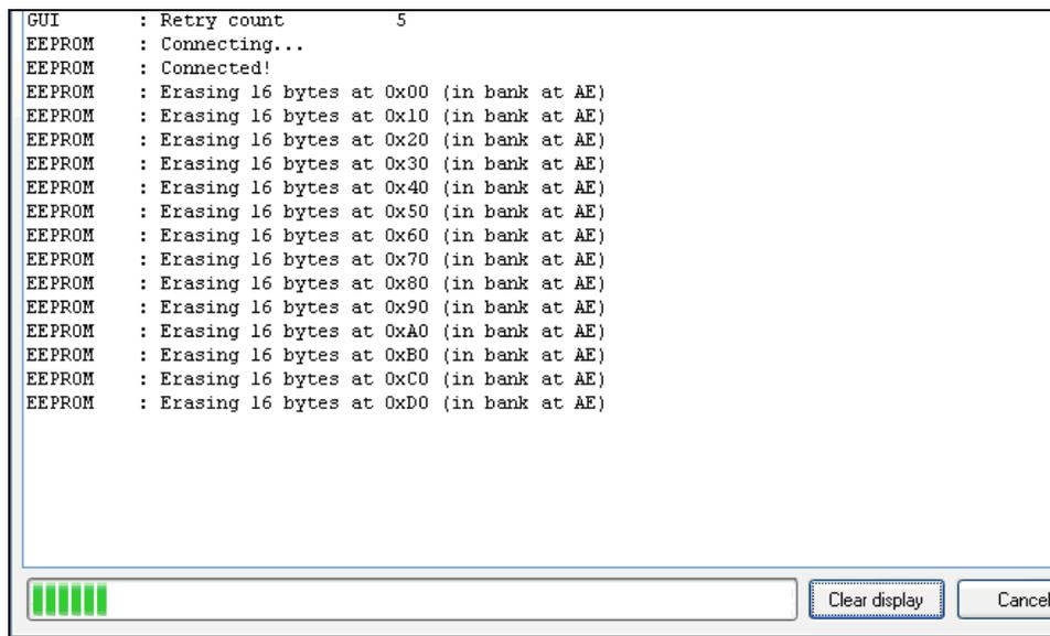
Clicking the *Erase* button or *Erase* from the *EEPROM* menu initiates a complete erasure of the EEPROM device by programming it with FF bytes. Before the erase operation begins the user is warned that the contents of the device will be changed and prompted to continue.
