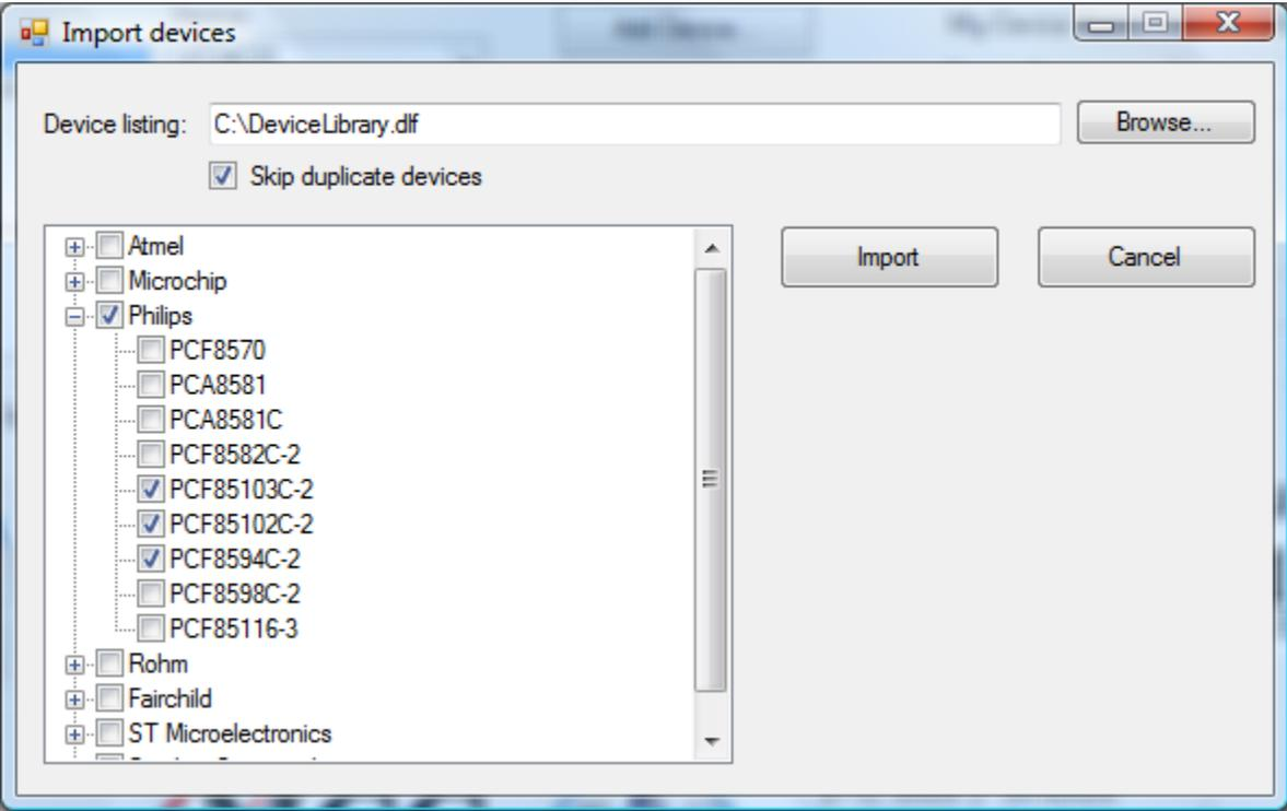
A complete device library that was previously exported or any selection of devices within it can be imported into iBurner by clicking the *Import Device...* button, or *Import device listing...* from the *Device Library* submenu of the *EEPROM* menu. Devices can be checked or unchecked to denote whether or not they will be imported. By default, no devices are checked. A device manufacturer can be checked or unchecked to check or uncheck all of the devices belonging to that manufacturer.
