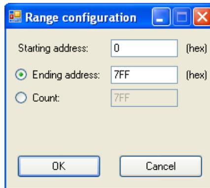
Clicking the *Read...* button or *Read...* from the *EEPROM* menu initiates a full or partial loading of data from the EEPROM into the buffer. The configuration window can be used to select the range to be loaded; the range defaults to the entire memory. Before a read operation begins the user is warned that the contents of the buffer will be changed and prompted to continue.
