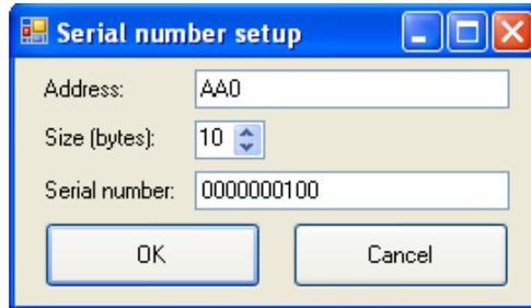
The address field is the hexadecimal address in the buffer where the serial number string should be inserted before each program operation. Enter the size of the serial number string, and the current value. You may now click the "Write serial number" checkbox in the program operation configuration dialog; the displayed serial number will be inserted into the buffer. Following the program operation the serial number will be incremented.
