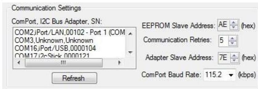
Use the *Communication settings* fields to configure the iPort. If necessary, click the *Refresh* button to have iBurner redetect available serial ports (including virtual serial ports provided by iPort/USB, iPort/LAN, and i2cStick devices). Select the serial port that corresponds to your device.
