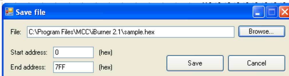
The buffer, or some portion thereof, can be saved to a file. As with loading files, binary, Intel Hex, and Motorola S-Record files are supported. The selected range to save defaults to the entire buffer.
