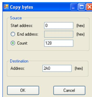
The *Copy* operation copies some portion of the buffer to a different location. The source and destination locations can overlap (eg. bytes 0 through 4 could be copied to bytes 1 through 5, if desired). The start address defaults to the address of the currently selected byte in the buffer; the end address (or count) and the destination address have no default value.
