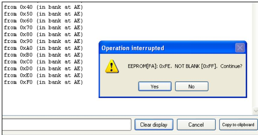
Clicking the *Blank check* button or *Blank check* from the *EEPROM* menu initiates a scan of the connected EEPROM to determine if the device contains any data (non-FF bytes). If such a byte is detected, the user is prompted to stop checking or continue. The information is logged as it is processed, including user decisions.
