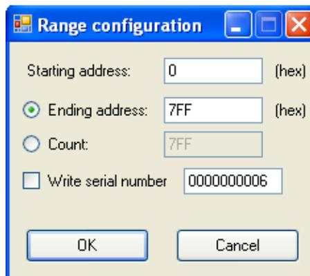
Clicking the *Program...* button or *Program...* from the *EEPROM* menu initiates a full or partial program of the connected EEPROM with data from the buffer. The configuration window can be used to select the range to be programmed; the range defaults to the entire memory. Before a program operation begins the user is warned that the contents of the EEPROM will be changed and prompted to continue.
