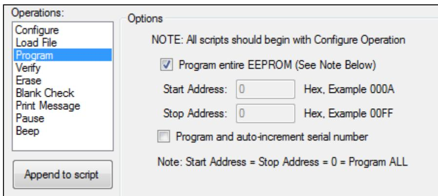
The “Program” operation programs a selected region of the EEPROM with the buffer, and optionally inserts a serial number into the buffer (and auto-increments it upon successful programming). The serial number configuration (size, initial value, and offset within the buffer) can be set in the main iBurner application.
