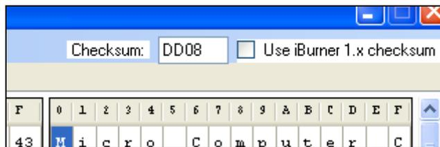
The *Buffer* tab displays the current checksum for the buffer in a text box at the top of the window. This checksum is a standard CRC16 computation (CRC polynomial A001) and can be used to quickly verify the contents of the buffer. To preserve compatibility with older versions of the iBurner software, the “Use iBurner 1.x checksum” checkbox may be checked; this is not recommended for use beyond backwards compatibility – the default CRC16 provides a more common and robust checksum.
