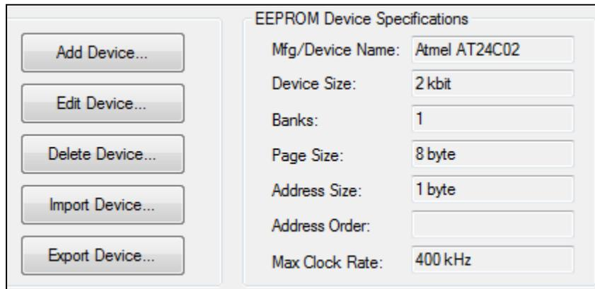
The screenshot shows a dialog box titled "EEPROM Device Specifications". On the left side, there are five buttons: "Add Device...", "Edit Device...", "Delete Device...", "Import Device...", and "Export Device...". On the right side, there are several input fields for device specifications:
