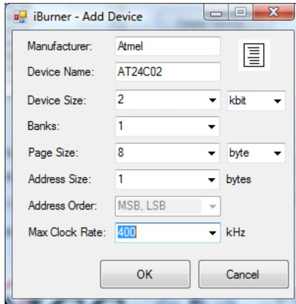
New device descriptions can be added to the device library by clicking the *Add Device...* button, or *New device...* from the *Device Library* submenu of the *EEPROM* menu. See the “*I<sup>2</sup>C EEPROMs*” section for information on determining the proper parameters to describe a particular device.
