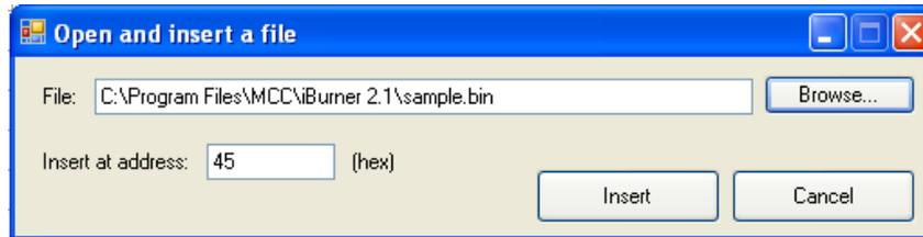
iBurner can load three types of files into the buffer: binary (or flat) files, Intel Hex files, and Motorola S-Record (S19) files. A binary file is any file that the user wishes to load byte-for-byte into the buffer. All files can be loaded with offsets: eg. a 128 byte binary file could be loaded into the buffer starting at address 0x70. The offset defaults to the address of the currently selected byte in the buffer.
