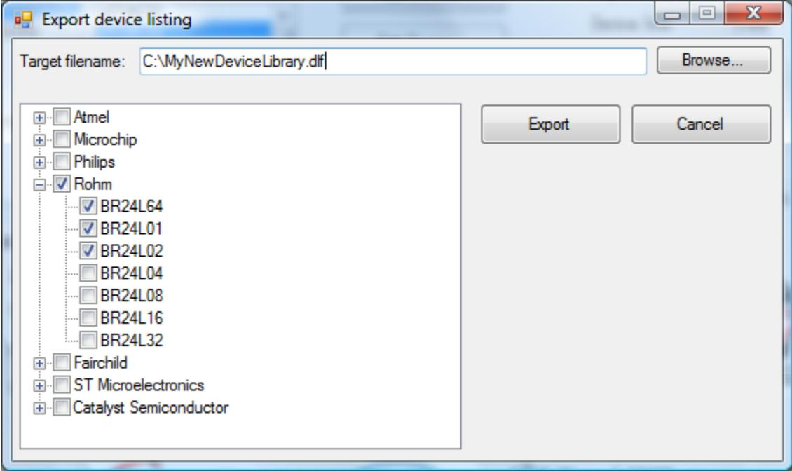
The complete device library or any selection of devices within it can be exported for use in another installation of iBurner by clicking the *Export Device...* button, or *Export device listing...* from the *Device Library* submenu of the *EEPROM* menu. Devices can be checked and unchecked to denote whether or not they will be exported. By default, no devices are checked. A device manufacturer can be checked or unchecked to check or uncheck all of the devices belonging to that manufacturer.
